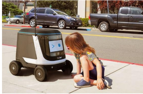
Figure 6. KiwiBot and the screen that shows the expression to get closer and interact with humans [21]
