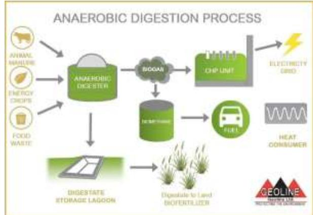
**Gambar 3.** Proses Anaerobic
