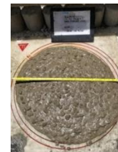
Gambar 6. Hasil Nilai Slump Trial Mix 2
