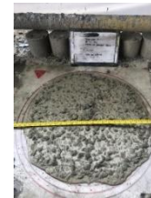
Gambar 5. Hasil Nilai Slump Trial Mix 1
