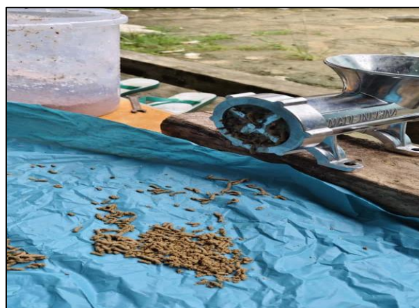
Figure 2. The Molding Process of the Fermented Alternative Feed
