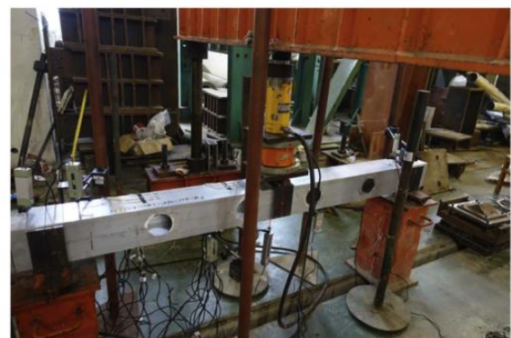
Gambar 4. Pengujian laboratorium skema three-point loading (Feng et al., 2017)
