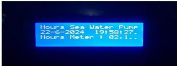
**Gambar 14.** Hasil Monitoring Pada LCD 20x4
