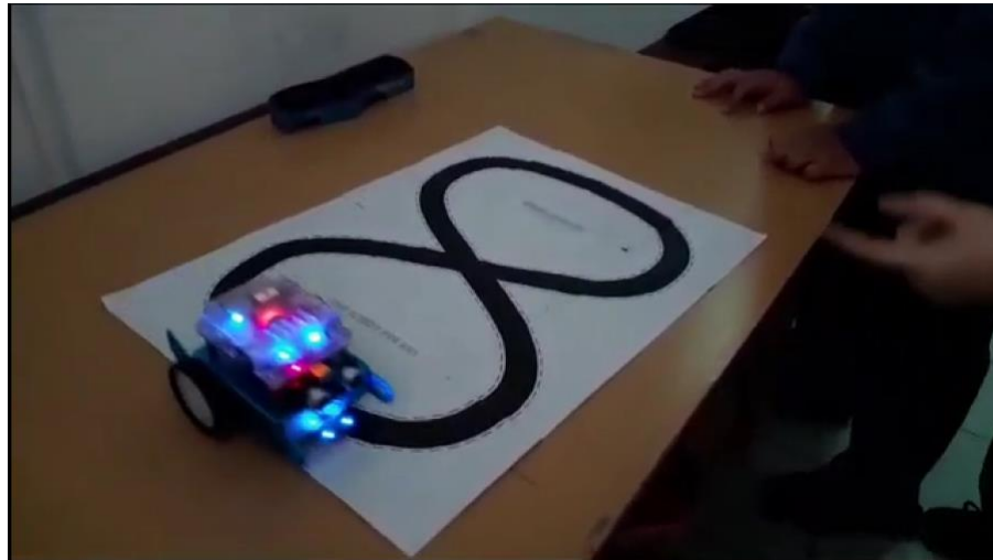
Gambar 5. Percobaan Sensor Line Follower
